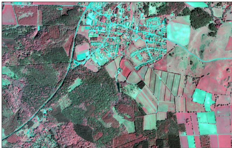
Figure 8 e: Infrared (NIR) digital colour aerial photograph 2010, 4600 m flying altitude, ground resolution approximately 0.25 metre
