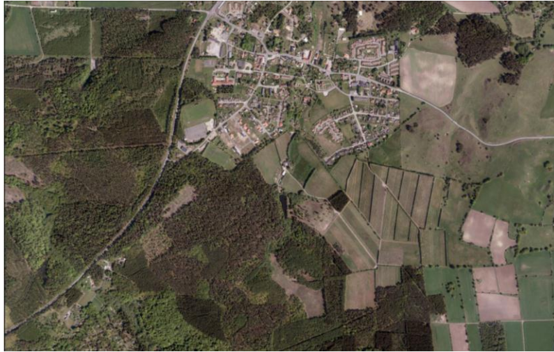
Figure 8 d: Colour digital aerial photograph 2010, 4600 m flying altitude, ground resolution approximately 0.25 metre
